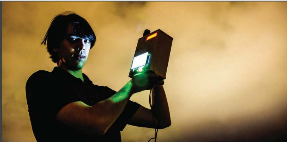
Naval Research Enterprise Internship Program (NREIP) student intern Julian Brown holds the star tracker system he developed during a summer in the university's Space Systems Academic Group. The low-cost star tracker is designed to help very small satellites determine their orientation in space.
