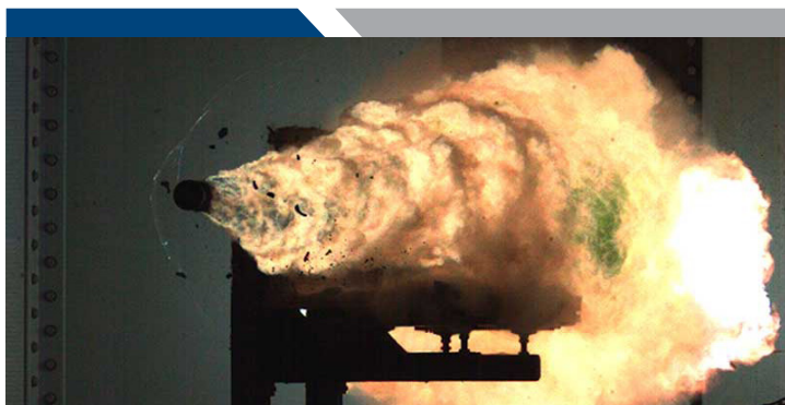
Advancements in railgun and hypervelocity projectile research since this 2008 test-firing at NSWC Dahlgren have led to promising operational possibilities. The concurrent development of NPS' capacity to teach and perform research in the tech space is producing alumni prepared to lead its development to the operational force. (U.S. Navy photo)
