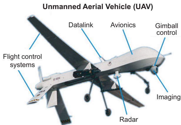
Fig. 4. Components of unmanned aerial vehicles (UAVs).
