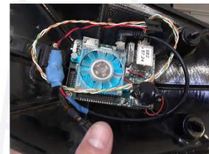
The secondary controller payload implemented the NPS autonomy architecture for cooperative ISR.
