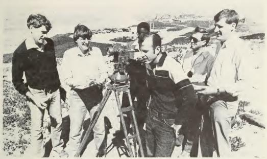
Mapping Charting and Geodesy students check out the operation of the wild T-3 optical theodolite used for precise positioning in hydrographic surveying
