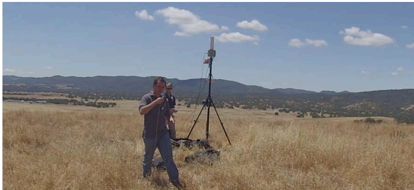
Setting up a mesh-network node using Persistent Systems Wave Relay Equipment. This, and other ad-hoc networks were used to move data from multiple locations to the Technical Operations Center during Data Integration Thursday.
