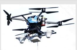
AT&T FlyingCOW (Cell on Wings) propagates 5G cellular signal.
