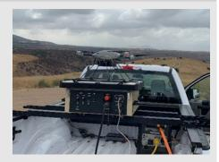
Planck Aerosystems vehicle-mounted tethered UAS.
