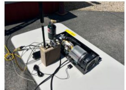
Configuration: LightCell, open, startup Result: little to no noise
