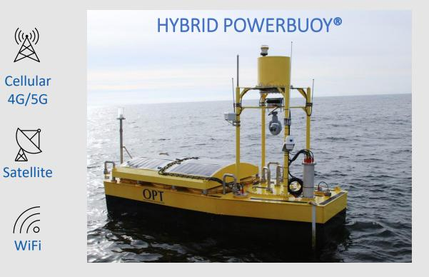
OPT's hybrid PowerBuoy<sup>®</sup> MSS solution, is powered by renewable solar power and efficient Stirling engine backup power and is designed for shorter deployments and lower wave energy environments.
