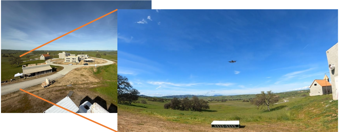
A-01: Reach Power kept their small UAS aloft through power beaming. The UAS is expected to fly for six minutes on its normal battery but remained aloft for over an hour through Reach’s power beaming technology.
