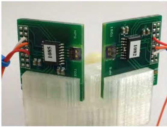
(A) (B) FIGURE 3. (A) DUAL SENSOR ASSEMBLY AND (B) MEASURED OUTPUTS OF THE TWO SENSORS AS A FUNCTION OF INCIDENCE ANGLE.
