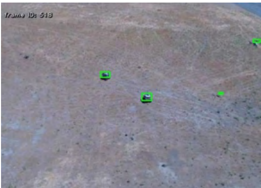
FIGURE 5. REAL-TIME DETECTION AND TRACKING OF MULTIPLE HETEROGENEOUS GROUND (A) AND AERIAL (B) TARGETS / THREATS [17].
