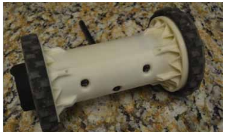
Figure 1. Robotic Research, LLC designed a 3D-printed ground robot for DHS, called TOSR (image is property of Robotic Research, LLC)
