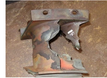
Turbine Vane with Hot Corrosion/ Oxidation: 4300 Hrs
