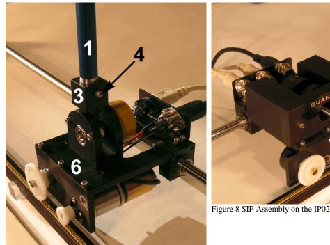
Figure 7 SIP Assembly on the IP01
