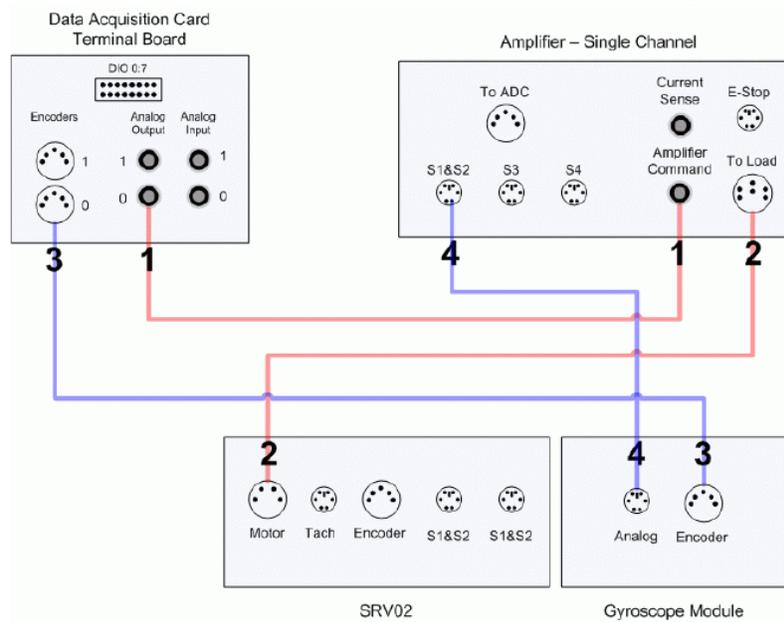
Figure 2. Schematic of SRV02 Gyroscope experiment.
