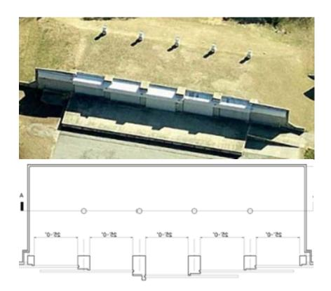
Figure A3. Picture and Layout of a Box D Magazine. Source: "Naval Ordnance" (2016).
