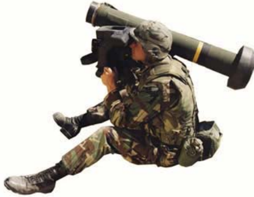
Figure 2. The Javelin Gunner Looks Through the Command Launch Unit (Lyons, Long, & Chait, 2006)
