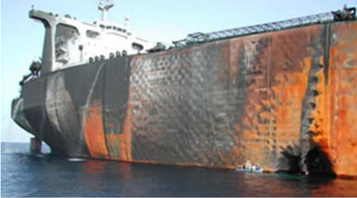
Figure 5. Damage to the French Tanker LIMBURG, October 2002
