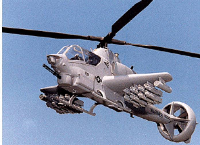
Figure XIV-8: Model of AH-1Z with vectored thrust ducted propeller and lifting wings (Source: Piasecki Aircraft, 1996)
