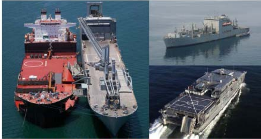
Mobile landing platform (MLP) moored with large, medium-speed roll-on/roll-off (LMSR) (left), auxiliary dry cargo ammunition (T-AKE) (top right), expeditionary fast transport (EPF) (bottom right).
