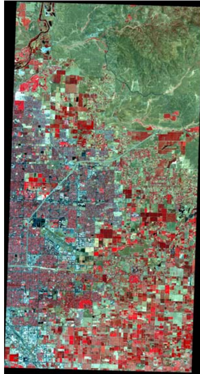
Figure 2. Quickbird data, nadir view, false-color IR image (bands 4,3,2) for the target area.
