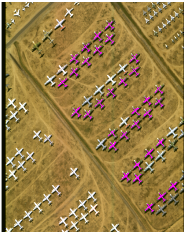
Figure 1. Subset of the boneyard from Davis Monthan AFB. This image is a 3-color composite formed by mapping HYDICE bands (48, 39, 13) corresponding to wavelengths of (636, 563, 441) (in nm) into the R-G-B display. The region concentrated on in this analysis corresponds to a set of C-130 aircraft painted with a standard camouflage pattern. There are 34 such aircraft. The pink pixels compose the ROI, and there are 1,740 pixels. One camouflaged aircraft is shown without the overlying ROI to differentiate the camouflaged pattern from the other aircraft.
