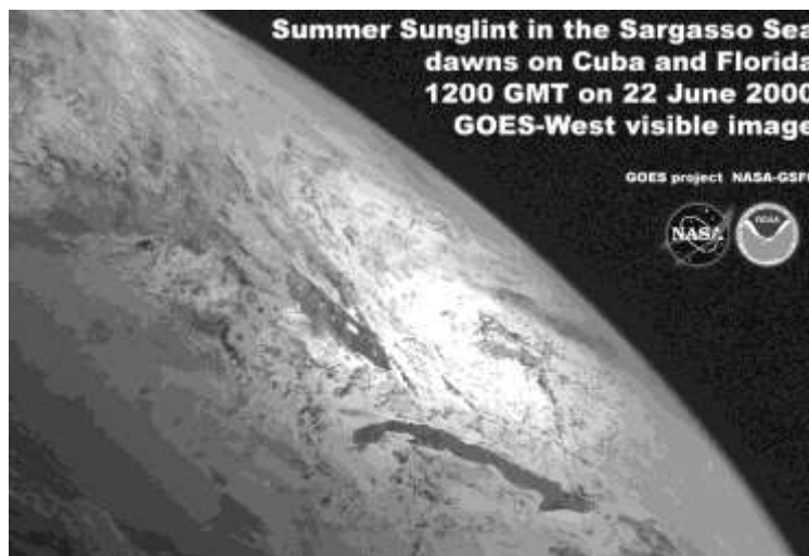
Figure 12. Another example demonstrating the effect of sun glint on the imager (image captured by the GOES satellite on 22 June 2000) (From http://rsd.gsfc.nasa.gov/goes/text/hotstuff.html )
