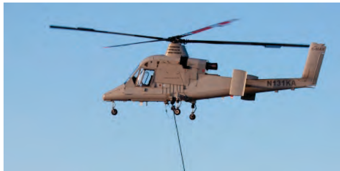
K-MAX FLIES AUTONOMOUSLY TO DELIVER CARGO TO REMOTE OUTPOSTS. PHOTO BY LOCKHEED MARTIN
