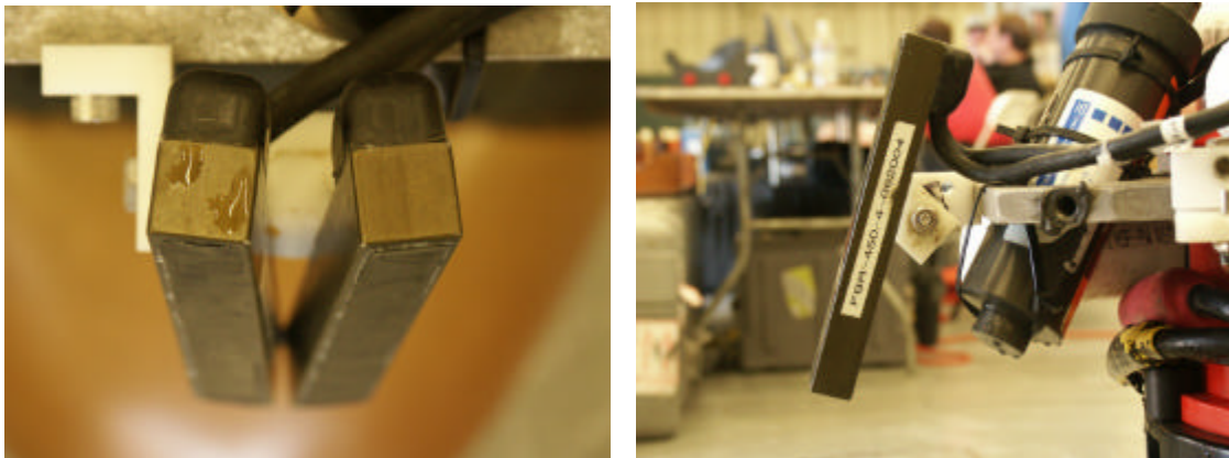
Figure 3 Blazed Array Vertical Configuration. Top View at Left, Side View at Right
