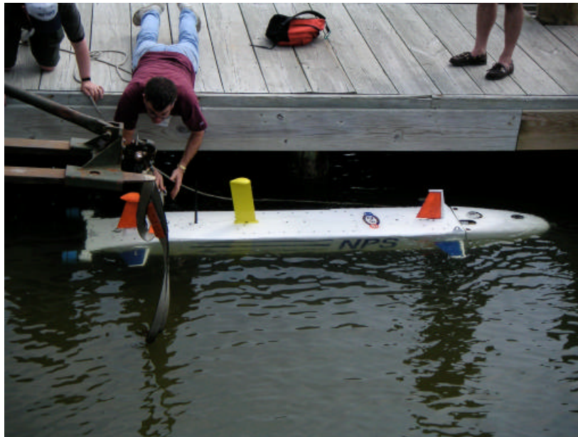
Figure 1. ARIES AUV Being Deployed at Camp Lejeune (Yellow Fin Carries 802.11b Antenna (1 Watt))
