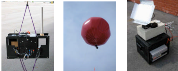
Figure 3 Balloon Payload Balloon and K2 Tracking Antenna
