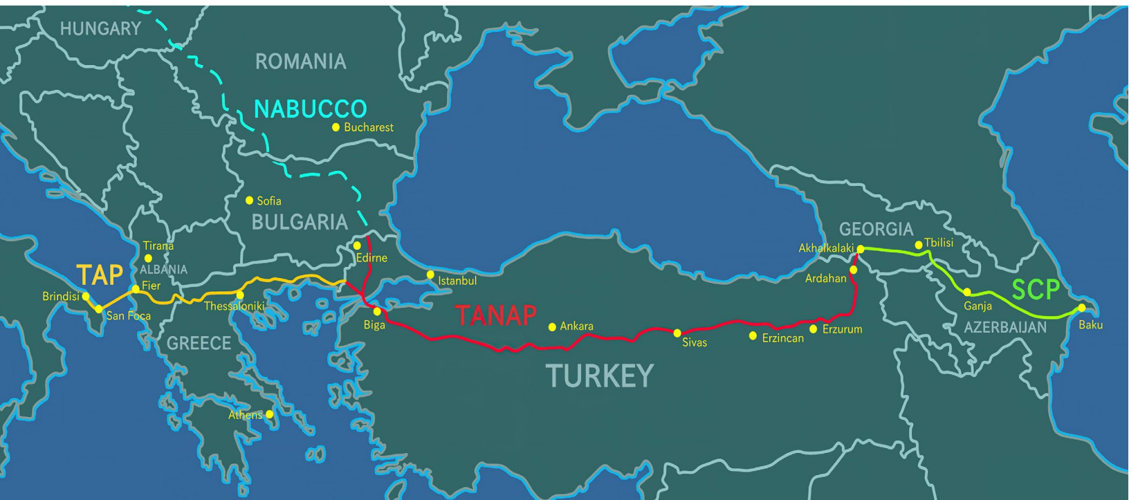
Map of the Southern Gas Corridor, consisting of Southern Caucasus pipeline (SCP), Trans-Anatolian gas pipeline (TANAP), Trans-Adriatic pipeline (TAP).
