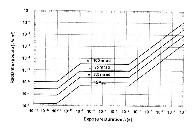
Figure 7. MPE for Ocular Exposure to Visible Laser Radiation (Wavelengths from 0.400 to 0.700 µm) for Single Pulses or Continuous Exposure (Small or Extended Sources)
