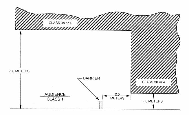
Figure 2c. Unsupervised Laser Installation for Demonstration Laser
