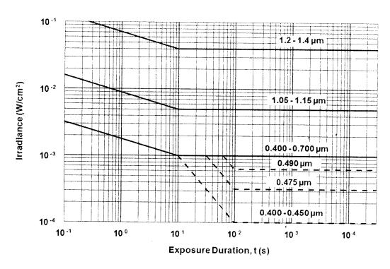
Figure 10a. Ocular Point Source MPE ( $\alpha \le 1.5$  mrad) for Visible and Near Infrared Laser Radiation (Wavelengths from 0.400 to 1.400  $\mu m$ ) See Table 5a.
