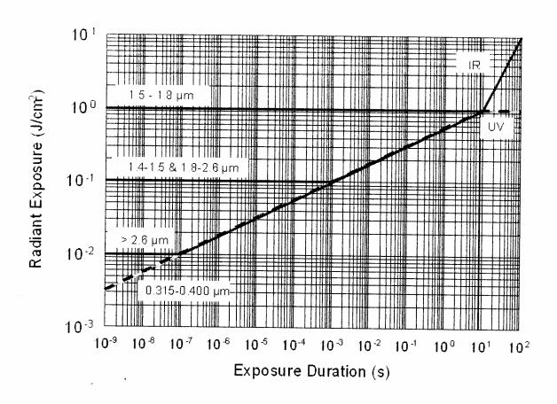
Figure 6. MPE for Ultraviolet (Wavelengths from 0.315 to 0.400  $\mu m)$  and Infrared Radiation (Wavelengths from 1.400  $\mu m$  to 1mm) for Single Pulses or Continuous Exposure (Small or Extended Sources)
