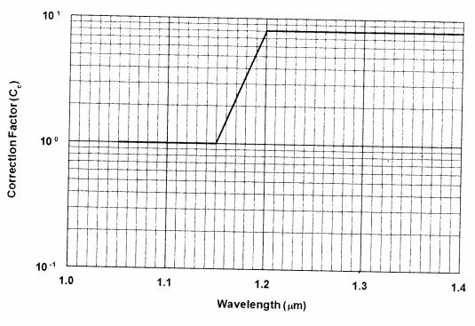
Note:  $C_{\rm C} = 1.0$  for  $\lambda = 1.050$  to 1.150  $\mu m$   $C_{\rm C} = 10^{18(\lambda - 1.150)}$  for  $\lambda = 1.150$  to 1.200  $\mu m$  $C_{\rm C} = 8$  for  $\lambda = 1.200$  to 1.400  $\mu m$
