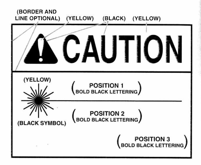
Figure 1a. Sample Warning Sign for Class 2 and Class 2M Lasers
