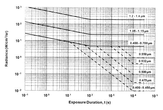
Figure 11. Ocular Extended Source MPE ( $\alpha \ge 110$  mrad) for Visible and Near Infrared Laser Radiation (Wavelengths from 0.400 to 1.400  $\mu$ m)
