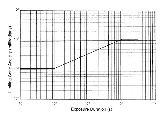
Figure 3. Limiting Cone Angle  $\gamma$ , Photochemical MPEs
