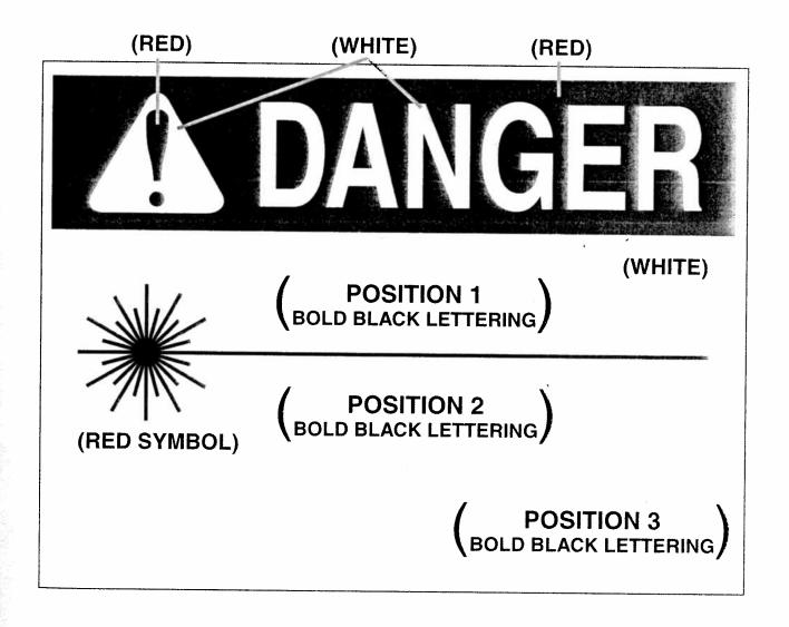
Figure 1b. Sample Warning Sign for Class 3R, Class 3B, and Class 4 Lasers
