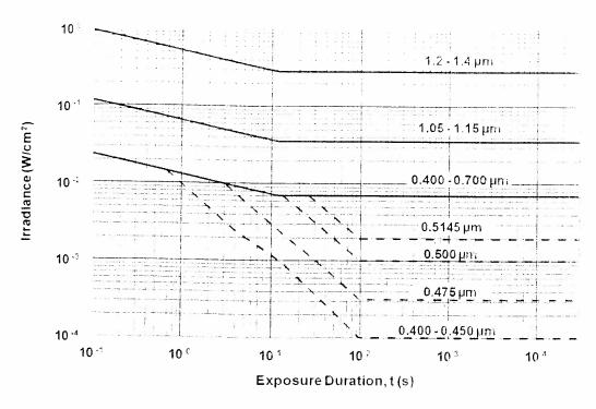
Figure 10c. Ocular Extended Source MPE ( $\alpha \leq 11$  mrad) for Visible and Near Infrared Laser Radiation (Wavelengths from 0.400 to 1.400  $\mu m$ ). See Table 5b.
