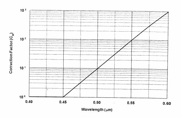
Figure 8c. Correction Factor  $C_B$  used to Determine the MPE for Wavelengths from 0.400 to 0.600  $\mu m$  See Table 6.
