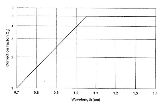
$C_{\rm A} = 1$  for  $\lambda = 0.400$  to 0.7.00  $\mu {\rm m}$   $C_{\rm A} = 10^{2(\lambda - 0.700)}$  for  $\lambda = 0.700$  to 1.050  $\mu {\rm m}$   $C_{\rm A} = 5.0$  for  $\lambda = 1.050$  to 1.400  $\mu {\rm m}$ Note:
