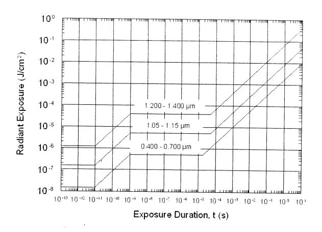
Figure 4. Point Source MPEs for Visible and Near Infrared Pulsed Sources (Wavelengths from 0.400 to 1.400  $\mu m)$
