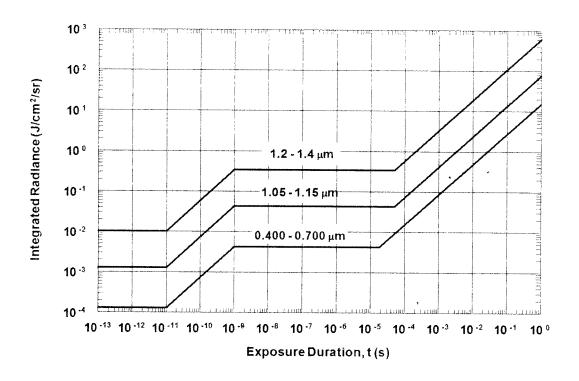
Figure 12. Ocular Extended Source Radiance MPE (α ≥ 100 mrad) for Visible and Near Infrared Laser Radiation (Wavelengths from 0.400 to 1.400 μm) for Pulsed or Continuous Exposures less than 1 s See Table 5b.
