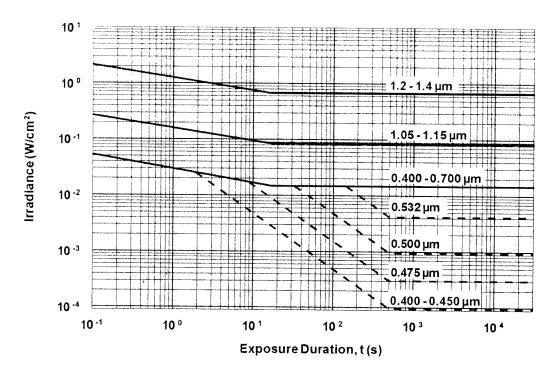
Figure 10d. Ocular Extended Source MPE ( $\alpha$  = 25 mrad) for Visible and Near Infrared Laser Radiation (Wavelengths from 0.400 to 1.400  $\mu$ m) See Table 5b.
