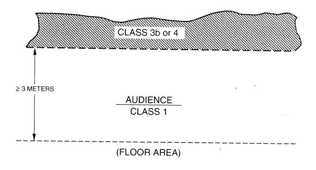
Figure 2d. Supervised Laser Installation for Demonstration Laser
