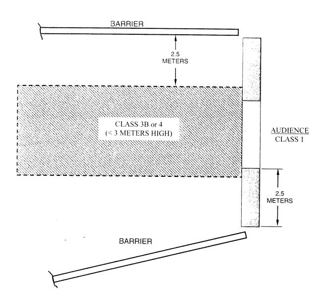
Figure 2e. Supervised Laser Installation for Demonstration Laser
