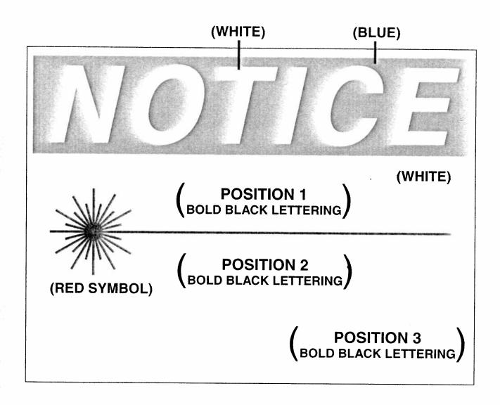
Figure 1d. Sample Warning Sign for Facility Policy, for example, Outside a Temporary Laser Controlled Area During Periods of Service
