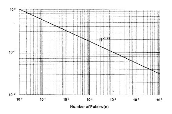
Figure 13. MPE Reduction Factor  $(C_P)$  for Repetitive-Pulse Lasers and Multiple Exposures from Scanning Lasers
