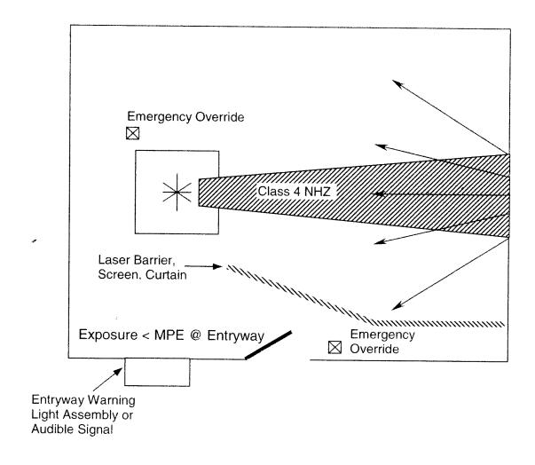
Figure 2b. Entryway Safety Controls for Class 4 Lasers without Entryway Interlocks
