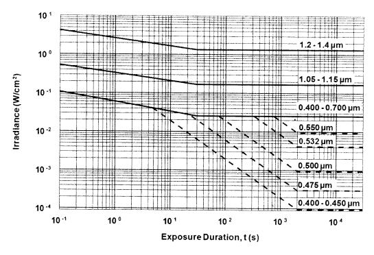
Figure 10e. Ocular Extended Source MPE ( $\alpha$  = 50 mrad) for Visible and Near Infrared Laser Radiation (Wavelengths from 0.400 to 1.400  $\mu$ m) See Table 5b.
