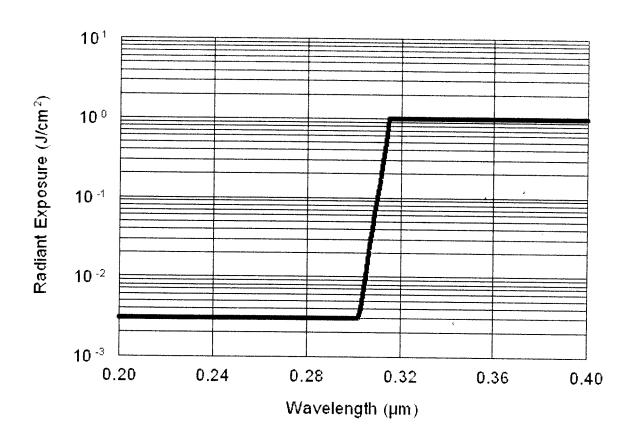
Figure 5. MPE for Ultraviolet Radiation (Small and Extended Sources) for Exposure Duration from  $10^{-9}$  to  $3\times10^4$  s for Ocular Exposure and  $10^{-9}$  to  $10^3$  s for Skin Exposure\*
