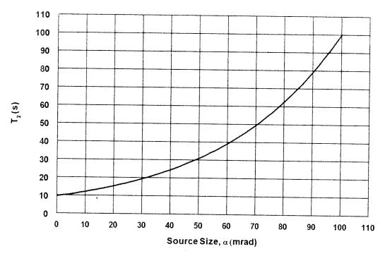
$T_2 = 10 \times 10^{(\alpha-1.5)/98.5}$  for wavelengths from 0.400 to 1.400 µm ( $\alpha$  is in milliradians)  $T_2 = 10$  s for point sources  $T_2 = 100$  s for sources equal to or exceeding 100 mrad
