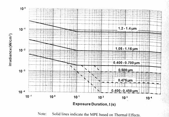
Dashed lines indicate the MPE based on Photochemical Effects.
