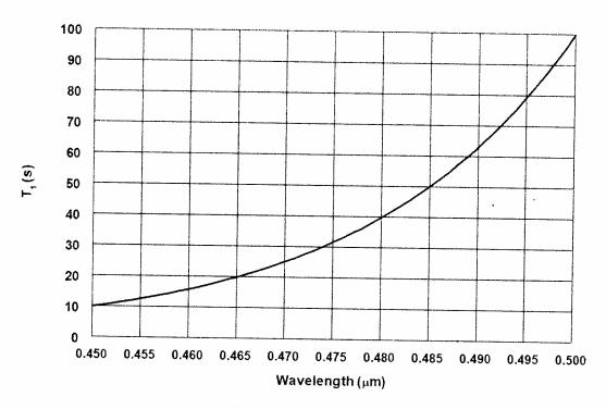
Note:  $T_1 = 10 \times 10^{20(\lambda - 0.450)}$  for wavelengths from 0.450 to 0.500 µm
