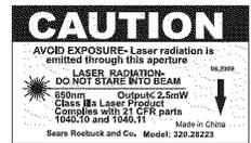
**⚠ WARNING: Laser light. Laser radiation.** Avoid Direct Eye Exposure. Do not stare into beam. Only turn laser beam on when the saw is on the workpiece. Class IIIa laser.
