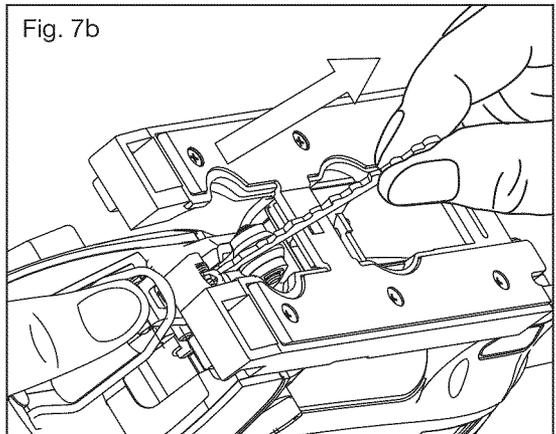
**⚠ CAUTION:** The blade guide rollers support the blade when cutting. The blade guide rollers must rest against the back of the blade. The ONLY cutting operation where the blade guide rollers do not support the blade is when the saw is in the scrolling mode. When scrolling, the blade must swivel as it is guided to follow the scroll pattern. Always move the base back and blade guide rollers up and back away from the blade when operating in scrolling mode. (Fig 8a, 8b)
