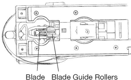
Fig. 8b Blade guide rollers up and back away from blade when operating in the scrolling mode.
