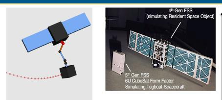
A Autonomous 6-U CubeSat Simulator (left) acts as tugboat-spacecraft of a RSO Simulator (right) during follow-on tests at the Spacecraft Robotics Lab
