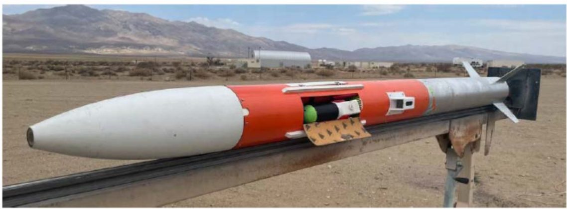
Figure 2: Rapid-response vehicle flight vehicle and exposed submunition on launch rail
