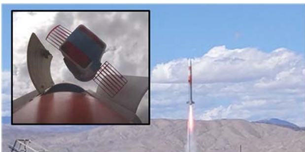
Figure 3: Launch of delivery vehicle with inset of submunition ejection at apogee
