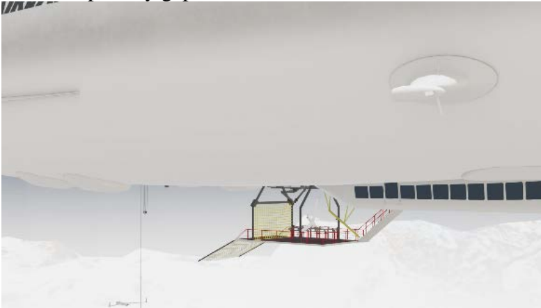
Figure 9: Platform view under Airlander 10 as ScanEagle is recovered. Source: NPS
