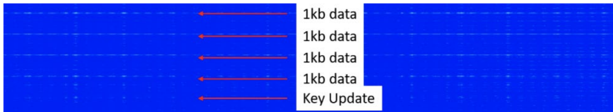
Figure 10: MLS test showing low radio frequency detectability for key updates
