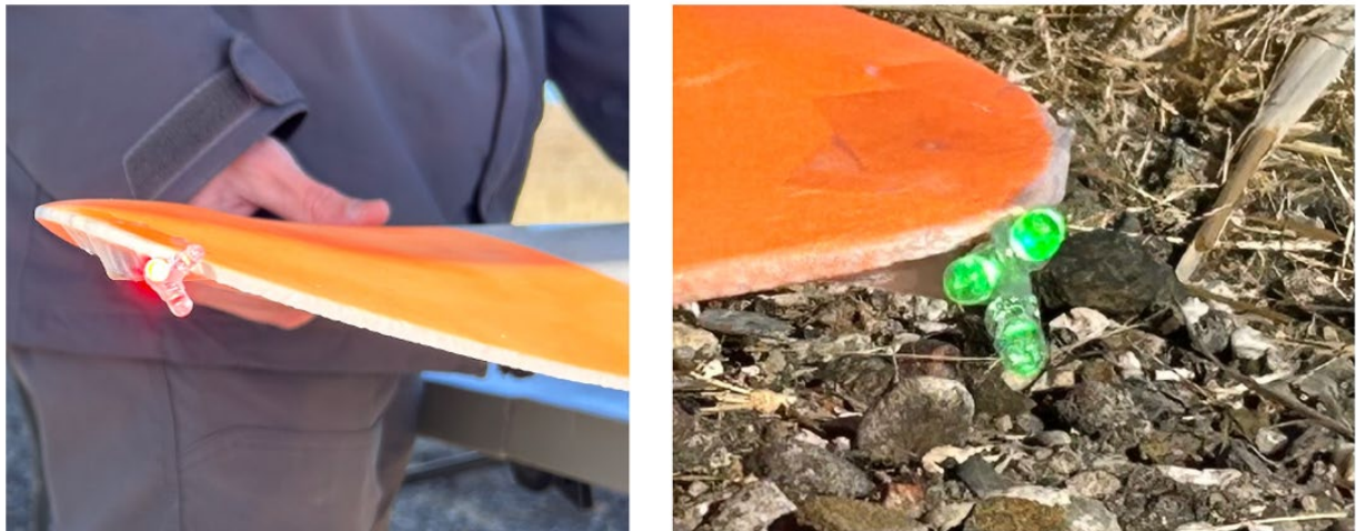
Figure 3: Wingtip LED clusters with 3 red LEDs on the left wingtip and 3 green LEDs on the right wingtip.
