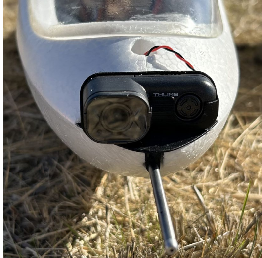
Figure 2: Redesigned camera mount shown with filter installed.
