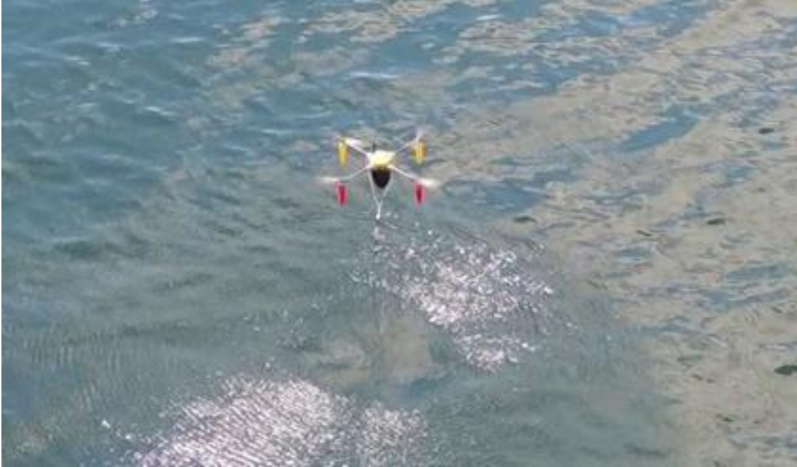
Figure 7: Aqua-Quad lifting off in Dabob Bay with the slung load still submerged
