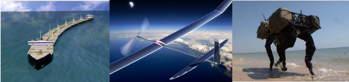
Figure 9. Proposed elements of the attritable communications and logistics system include the modular Sea Train USV 7 (left), a solar powered UAV glider 8 (center), and the Big Dog UGV 9 (right).
