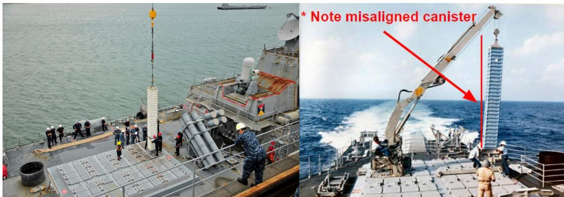
Figure 28. Current VLS reload in port 18 (left) and underway (right).
