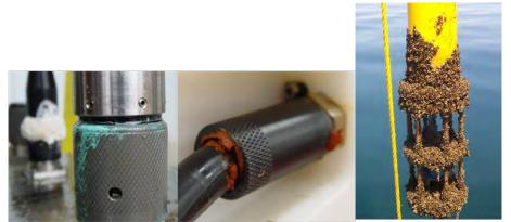
Figure 12. Corrosion<sup>5</sup> (*left*) and biofouling<sup>6</sup> (*right*) are common causes of sensor failure.
