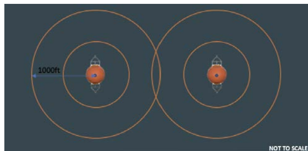
Figure 32. Buoy sensor network proposed two-way communications via a 5G mm mobile ad-hoc network, and LOS for communications within a 1000ft range (graphic representation not to scale).
