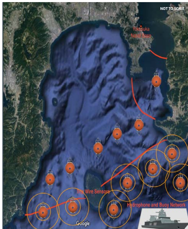
Figure 35. Undersea Buoy Sensor Grid would be placed between 3 and 12 NM from port ( not to scale ).
