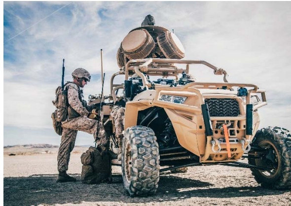
Figure 40. Land-based systems such as this light marine air defense integrated system (LMADIS) as part of a human-machine team are a component of the deployable Sensor Network SoS.
