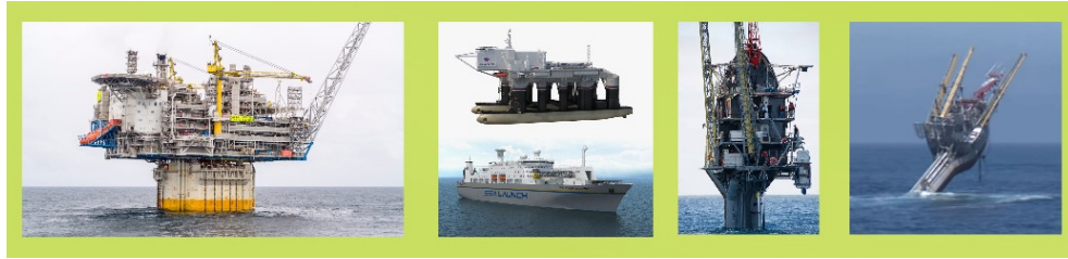
Figure 18. Mobile sea base frame options include spar platform ( left ), catamaran ( center ), or "flip ship" ( two at right ).
