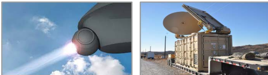
Figure 30. Aerostat payload package would include SAR, EO/IR, MAD, HEL ( left ), and high-power microwave technology.
