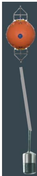
Figure 34. Individual buoy sensor, a hydrophone extended down to the seafloor tethered to a buoy, intended to be deployed throughout a battlespace to form the Undersea Buoy Sensor Grid.
