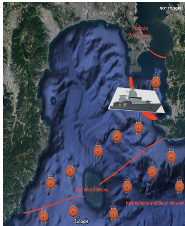
Figure 36. Seafloor cables placed at different distances from a port comprise the Trip Wire concept, and work in conjunction with the Undersea Buoy Sensor Grid and the Buoy Sensor Network.
