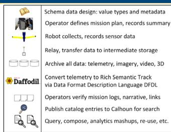
*Robodata Workflow: collection and storage of data enables recording, replay, smoothing and visualization of robot tracks.*
