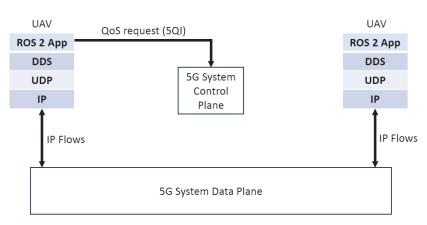
System Architecture that includes two UAVs running the ROS2 application, communicating over the 5G control and data planes. Adapted from https://design.ros2.org/articles/unique\_network\_flows.html
