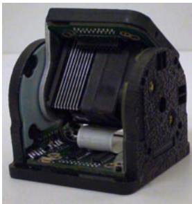
(a) A CKBot UBar module
