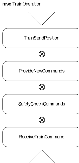
Fig. 7. TrainOperation HMSC for the BART specification
