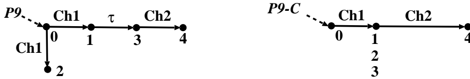
Figure 4: Example of IOT-states and IOT-state equivalent MLTSs.
