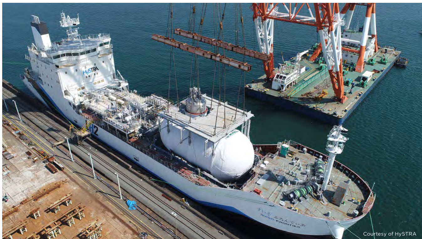
Figure 15: The Suiso Frontier is the First Liquid Hydrogen Carrier, Launched in 2019 and Intended for Use in the HESC Pilot Project
