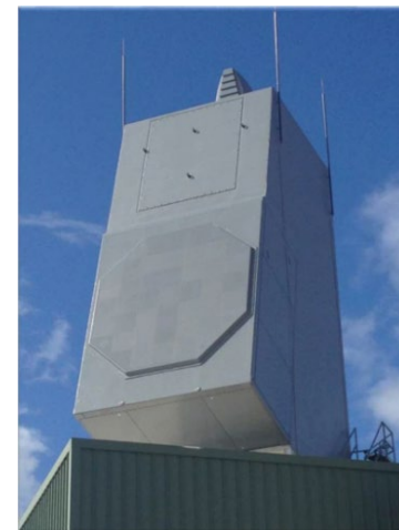
SPY-6 AMDR Radar, Credit Naval Sea Systems Command
