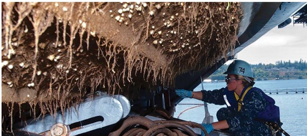
Fouling on Underside of USN Combatant Craft, Credit National Defense Magazine
