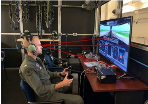
Normobaric Hypoxia Trainer Pilot Training Station with Notional Eye Tracking Range
