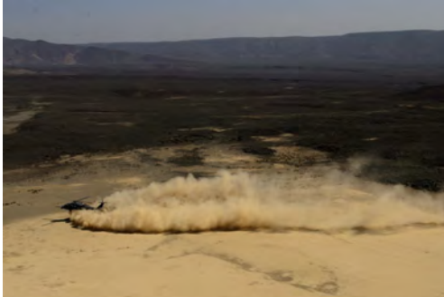
CAMP LEMONNIER, DJIBOUTI. A 303rd Expeditionary Rescue Squadron HH-60 Pave Hawk practices brownout landings near Camp Lemonnier, Djibouti, March 22, 2014. Brownout occurs when the rotor wash causes dirt, dust or sand to become airborne which can cause the crew to lose sight of the ground. (U.S. Air Force photo by Staff Sgt. Staci Miller/RELEASED).
