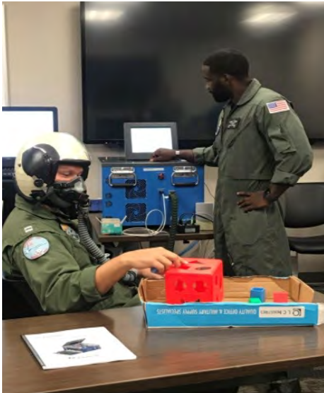
Engineering testing of On-Demand Hypoxia Trainer with Aerospace Physiologists at NAS Pensacola to validate pressure on demand and initial training profile for hypoxia training.
