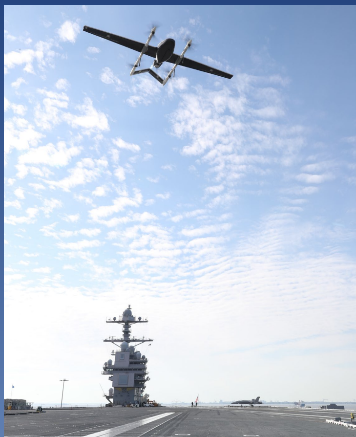
A logistics unmanned air system (UAS) prototype, called Blue Water UAS, approaches to deliver cargo on the USS Gerald R. Ford's (CVN 78's) flight deck during a Feb. 21 supply demonstration. (U.S. Navy)
