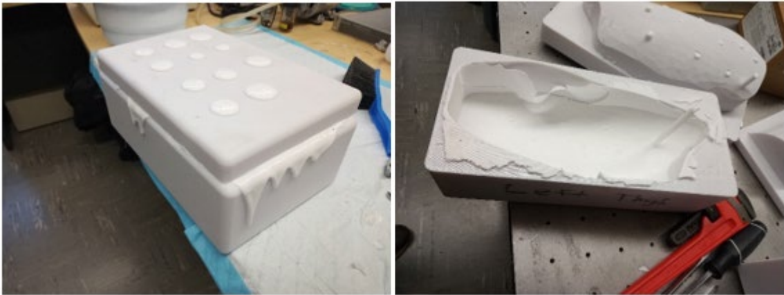
Figure 20. Molds Filled with Considerably more Mixture than Necessary.
