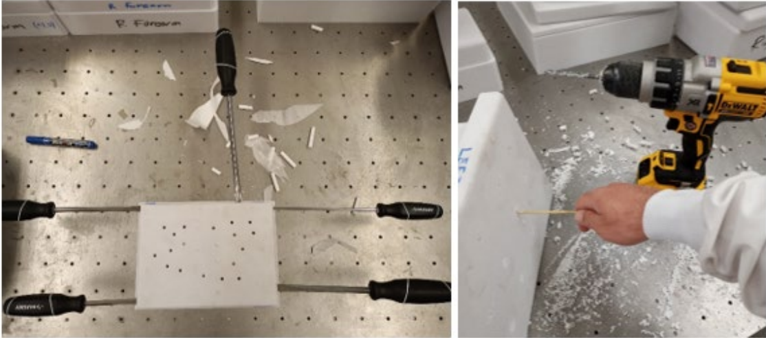
Figure 21. Removing the Lid from the Mold with the Use of Screwdrivers (left). Cleaning Excessive Debris from the Mold with the Use of a Drill and a Wooden Stick (right).
