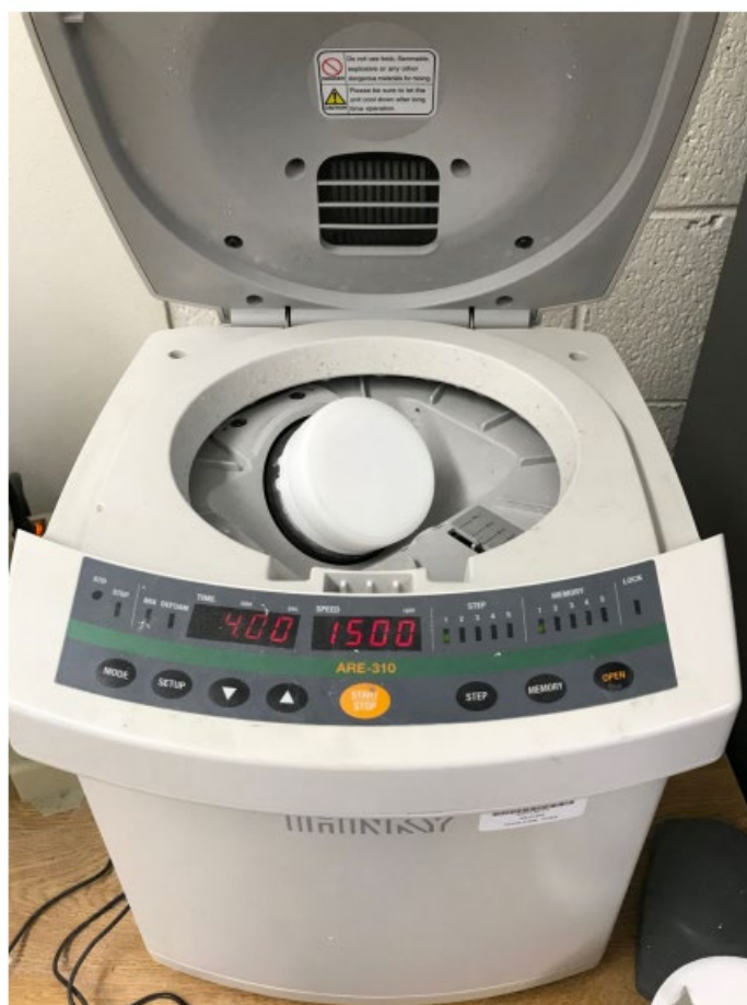
Figure 18. Cup with Composite Mixture in a THINKY Rotary Mixer Preset for Four Minutes Spinning at 1500 rpm. Source: [15].
