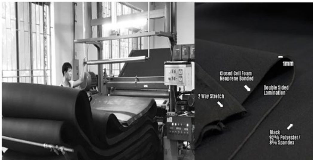
Figure 12. Manufacturing Neoprene Sheets (left). Source: [48]. 1mm Thickness Neoprene Sheet with Double Sided Lamination (right). Source: [49].
