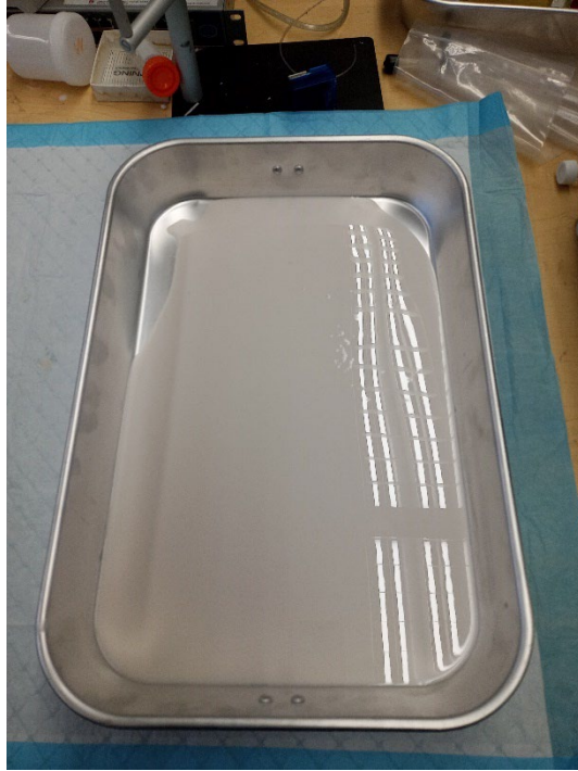
Figure 23. Ceramic Microspheres Mixture Poured in a Pan.
