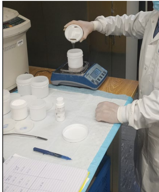
Figure 17. Mixing the PDMS Elastomer Base with the Curing Agent in a 310 mL Mixing Cup, on a Highly precise weight scale.
