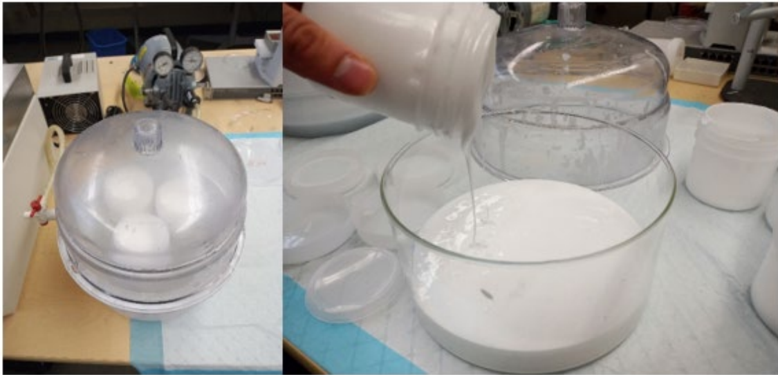
Figure 19. Degassing Three Cups with Mixture in a Desiccator Connected to a Mechanical Vacuum Pump (left). Pouring Glass Microspheres Mixture from a Cup to a Pyrex Bowl (right). Source: [28].
