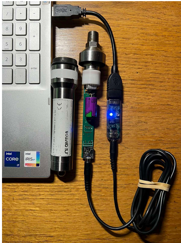
Figure 27. Connecting Data Logger to a USB Port.
